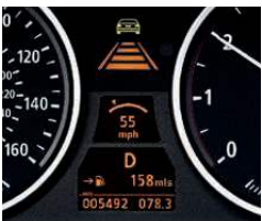
Active Cruise Control (ACC) with Stop & Go 3 allows the driver to preset both a desired speed and distance. When ACC recognizes slower vehicles ahead, it reduces your speed to maintain the preset distance. Stop & Go can bring you to a complete stop if traffic calls for it. When you press the accelerator, ACC resumes your speed according to your presets.
