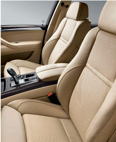
20-way power Multi-contour front seats conform to your body to provide optimum support and exceptional comfort over long distances. In addition to horizontal, vertical and angled adjustments, Multi-contour seats include an articulated upper backrest, backrest width, Comfort headrest (two-way power, two-way manual "relax headrest"), and four-way power-adjustable lumbar support. Both driver's and front-passenger's seats include memory function.
