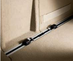
Storage package (included in Premium Package) adds a storage box under the front center console; safety-belt pretensioners for left and right rear seats (not included with optional third-row seating); in the cargo area, two lashing rails with four lashing points.
