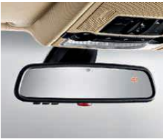
Automatic-dimming interior and exterior mirrors sense the bright headlights of vehicles behind you, and automatically darken. Includes fold-in function for exterior mirrors. Alarm system emits an acoustic signal and immediately switches on the hazard warning lights in the event of an attempted break-in or tampering.
