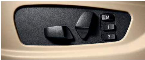
Power seat adjustment for driver and front passenger, with memory function for driver's seat, steering column and power-folding exterior mirrors.
