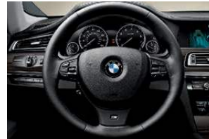
Three-spoke leather-wrapped multi-function M sport steering wheel features a slightly smaller diameter, thick padding, and special thumb rests for a comfortable grip during sporty driving maneuvers.
