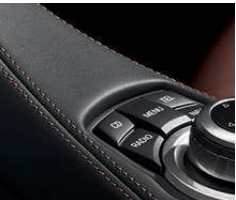
Contrast stitching is included with the extended Black Nappa Leather instrument panel, door and side trims, and center console. Two distinctively stitched flat-felled seams of the same color as the Nappa Leather upholstery add a custom effect to the instrument panel to embellish the interior. Contrast stitching for Black Nappa Leather upholstery is Gray.
