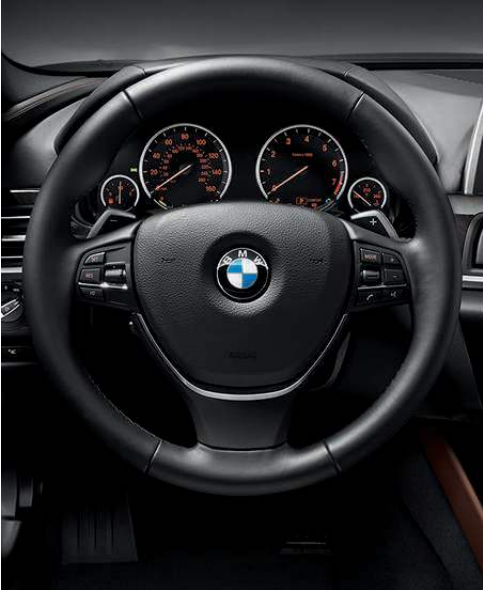
Three-spoke leather-wrapped multi-function sport steering wheel , featuring power tilt/telescoping adjustments, lets you keep both hands on the steering wheel while adjusting the audio, as well as your BMW-tested, Bluetooth ® enabled mobile phone. 3 The left-hand buttons operate all Cruise Control functions, while those on the right control audio functions, such as the radio, your mobile phone and Voice command.
