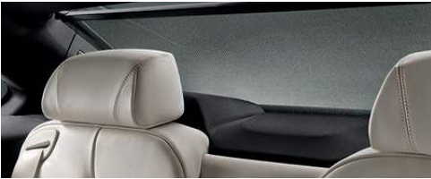
Power rear sunshade can be extended with the touch of a button to protect the Coupe's cabin from the sun's rays in warm weather, or retracted to allow the sun to help warm the interior in colder weather.
