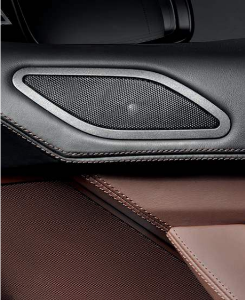
Premium anti-theft AM/FM stereo CD/MP3 audio system with Radio Data System (RDS), Auto-Store, and 3-channel FM diversity antenna. The Coupe's 16 speakers and the Convertible's 12 speakers feature DIRAC signal processing and Surround mode, and discrete 5.1 multi-channel sound. The 7-band equalizer incorporates an analog amplifier with vehicle-specific equalizing; it outputs 600 watts in the Coupe and 500 watts in the Convertible.
