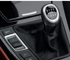
6-speed manual transmission delivers a precise, athletic feel. Its responsiveness is due, in part, to the synchronization of shifts from neutral to each gear. The shortened shift lever and "throw" add to the sporty feel of the gearbox. The sixth gear drops revs at highway speeds for smooth cruising and better fuel economy.
