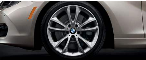
V Spoke (Style 366) 19 x 8.5 front, 19 x 9.0 rear light alloy wheels with 245/40 front and 275/35 rear run-flat 1 performance tires 2
