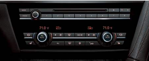
2-zone automatic climate control allows driver and front passenger to select individual temperatures and choice of fan speeds, as well as choose automatic or manual airflow and recirculation. The automatic recirculation control activates whenever certain air pollutants are detected. The system also offers a mist-up sensor, solar sensor and residual heat use.
