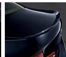
M rear spoiler complements the Sedan's sporty looks and also serves to increase rear-vehicle downforce at higher speeds.
