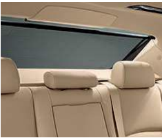
Power rear sunshade can be extended with the touch of a button to protect the cabin from the sun's rays in warm weather or retracted to allow the sun to help warm the interior in colder weather.
