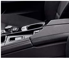
Front armrest with integrated storage compartment opens up to allow access to the iPod® and USB adapter, and Smartphone Integration adapter.
