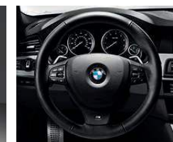
Three-spoke, leather-wrapped multi-function M sport steering wheel includes a thick, textured rim and thumb indents that are designed for performance driving. Multi-function buttons allow you to adjust various comfort features while keeping both hands on the wheel.
