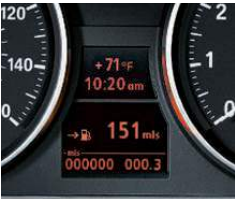
The on-board computer with Check Control provides valuable feedback on the vehicle's operating status: oil level indicator and distance to next service appointment/oil change, as well as other detailed information, such as spark plug and micro-filter status. It also provides travel information: travel range on remaining fuel, external temperature and more.
