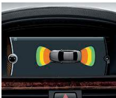
Park Distance Control uses ultrasonic sensors in the front and rear bumpers to help you judge the distance to other vehicles and unseen objects when parking. While parking, the image on the screen visually changes and warning beeps come faster as your bumper approaches a stationary object, turning into a constant tone when the distance is less than 12 inches.
