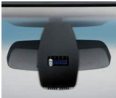
Rain sensor uses infrared light to measure the amount of falling rain and spray from other vehicles. When the wipers are in the "intermittent" mode, the rain sensor automatically adjusts the windshield wiping interval as needed. Automatic headlight control activates headlights by means of a sensor that responds to darkness.
