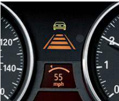
Active Cruise Control (ACC) with Stop & Go 1 allows the driver to preset both a desired speed and distance. When ACC recognizes slower vehicles ahead, it reduces your speed to maintain the preset distance. Stop & Go can bring you to a complete stop if traffic calls for it. When you press the accelerator, ACC resumes your speed according to your presets.
