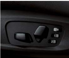
■/❑ Power seat adjustments included with eight-way power front seats allow customized comfort and convenience for driver and front passenger. The two-setting memory system automatically adjusts the driver's seat and side-view mirror positions, with individual preferences available at your fingertips.
