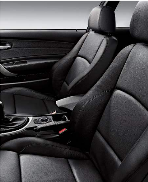
❑ Eight-way adjustable front sport seats , included in the Sport Package or M Sport Package, make the driving experience more enjoyable. Side bolsters can be power-adjusted to fit your back comfortably while helping to hold you firmly in place during tight cornering. Includes two-way headrests and thigh support for added support. (Shown with optional Black Boston Leather upholstery and iDrive.)
