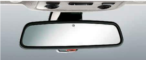
❑ Automatic dimming interior and exterior mirrors respond to the brightness of following headlights to minimize their reflection in the eyes of the driver. The automatic anti-glare function improves safety and comfort when driving at night by helping to eliminate the eye strain from excess glare. The digital compass, integrated into the mirror, is a convenient way to constantly keep your bearings while driving. Both power-adjustable exterior mirrors include a fold-in function. The passenger-side mirror folds down to reveal the curb when the transmission is shifted into reverse gear to back up.
