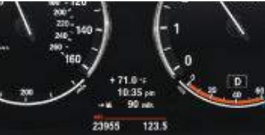
As soon as you brake or lift your foot off the throttle, Brake Energy Regeneration converts the braking energy released by the vehicle into electric power, and feeds it into the battery. The charge process is displayed by a symbol in the tachometer.
