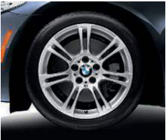
Double Spoke (Style 350M) 18 x 8.0 front, 18 x 9.0 rear light alloy wheels with 245/45 front and 275/40 rear run-flat 1 performance tires 2 .
