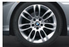
□ Double Spoke (Style 195) light alloy wheels and run-flat 1 performance tires 2 . In front: 18 x 8.0 wheels and 225/40 tires; in back: 18 x 8.5 wheels and 255/35 tires. (Included in 335d Sport Package.)
