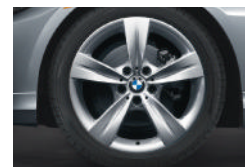
□ Star Spoke (Style 287) light alloy wheels and run-flat 1 performance tires 2 . In front: 18 x 8.0 wheels and 225/40 tires; in back: 18 x 8.5 wheels and 255/35 tires. (Included in 335i Sport Package; optional on 335i xDrive, requires optional Sport Package.)
