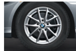
■ V Spoke (Style 360) 16 x 7.0 light alloy wheels with 205/55 run-flat 1 all-season tires . (Standard on 328i/328i xDrive.)
