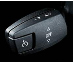
■ Dynamic Cruise Control lets you store and maintain a chosen speed above 20 mph. It is activated via the left-hand steering column switch, and deactivated by applying the brakes or via the switch. 2
