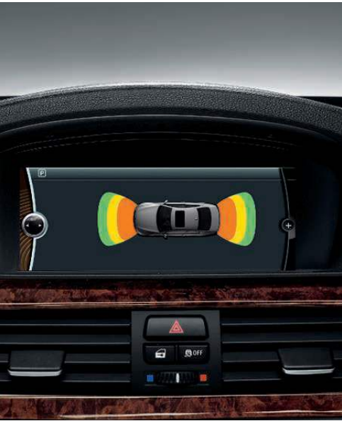
□ Park Distance Control uses ultrasonic sensors in the front and rear bumpers to help you judge the distance to other vehicles and unseen objects when parking. While engaged in a parking maneuver, the image on the screen visually changes and warning beeps come faster as your bumper approaches a stationary object, turning into a constant tone when the distance is less than 12 inches.
