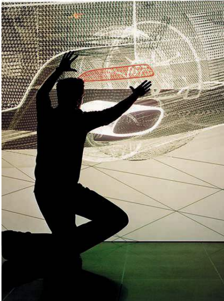
The projection screen (top) shows, with minute precision, what a future vehicle will look like. Details can be enlarged to any desired magnification.
