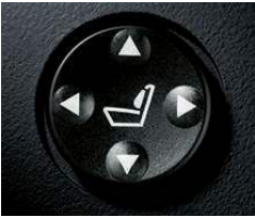
Lumbar support for front seats adds four-way adjustable comfort for the lower back. The up/down and in/out lumbar support positioning is electrically adjustable.
