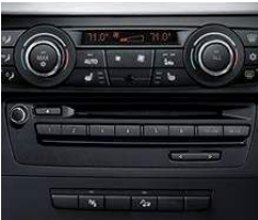
Memory buttons provide access to the most frequently used functions of the iDrive system. The six convenient buttons allow the driver and front passenger to store and then easily access any functions of the Navigation system; the audio system – including specific radio stations or CD tracks; and the Bluetooth® enabled mobile phone (if so equipped).
