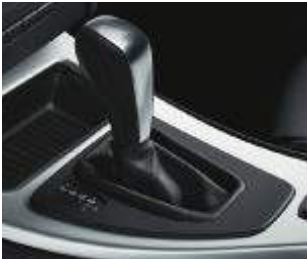
□ 6-speed STEPTRONIC automatic transmission provides a choice of three modes: “Drive” with Adaptive Transmission Control, “Sport” and STEPTRONIC automatic, for manual control without a clutch. Steering wheel-mounted paddle shifters are automatically added when ordered with Sport or M Sport Package.
