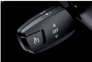
■ Cruise Control lets you store and keep to a chosen speed above 20 mph. It is activated via the left-hand steering column switch and deactivated by applying the brakes or via the switch. (Cruise Control is not a substitute for the driver's own responsibility in adjusting speed and otherwise controlling the vehicle. Due to road, traffic and visibility conditions, the driver decides whether and how the system is used.)
