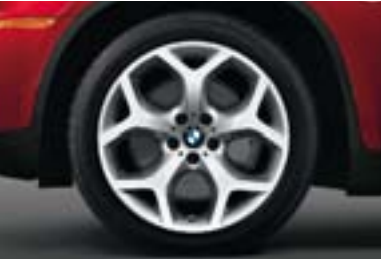
Y Spoke (Style 214) 20 x 10.0 front, 20 x 11.0 rear light alloy wheels with 275/40 front and 315/35 rear run-flat 1 performance tires 2 are available as an option when ordering the X6 xDrive35i Sport Package and Sport Activity Package. (Not available on X6 xDrive50i.)
