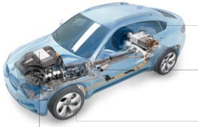
Electric air conditioning compressor: The electric drive of the air conditioning system runs independently of the combustion engine. You can create a comfortable climate and maintain it while driving on electric power alone – or even when the engine is switched off. This leaves more hybrid energy available for other uses, and full use of all hybrid functions – even during sporty driving and in extreme weather.
