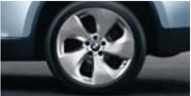
Streamline (Style 297) 20 x 10.0 front, 20 x 11.0 rear light alloy wheels with 275/40 front and 315/35 rear run-flat performance tires , 1 standard on the ActiveHybrid X6, reduce unsprung weight for increased performance.
