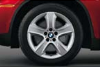
Star Spoke (Style 212) 19 x 9.0 light alloy wheels with 255/50 run-flat 1 all-season tires are included in the X6 xDrive35i Sport Package and Sport Activity Package. (Not available on X6 xDrive50i.)
