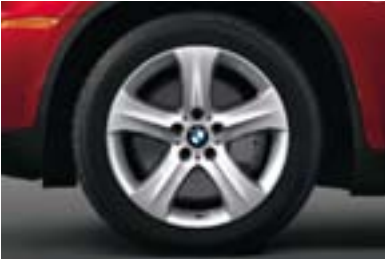
Star Spoke (Style 258) 19 x 9.0 light alloy wheels with 255/50 run-flat 1 all-season tires are included in the X6 xDrive50i Sport Package and Sport Activity Package. (Not available on X6 xDrive35i.)
