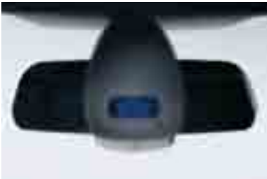
■ Rain sensor uses infrared light to measure the amount of rain. When the wipers are in the intermittent mode, the rain sensor automatically adjusts the windshield-wiping interval as needed. Automatic headlight control (not shown), included with rain sensor, activates headlights by means of a sensor that responds to darkness.
