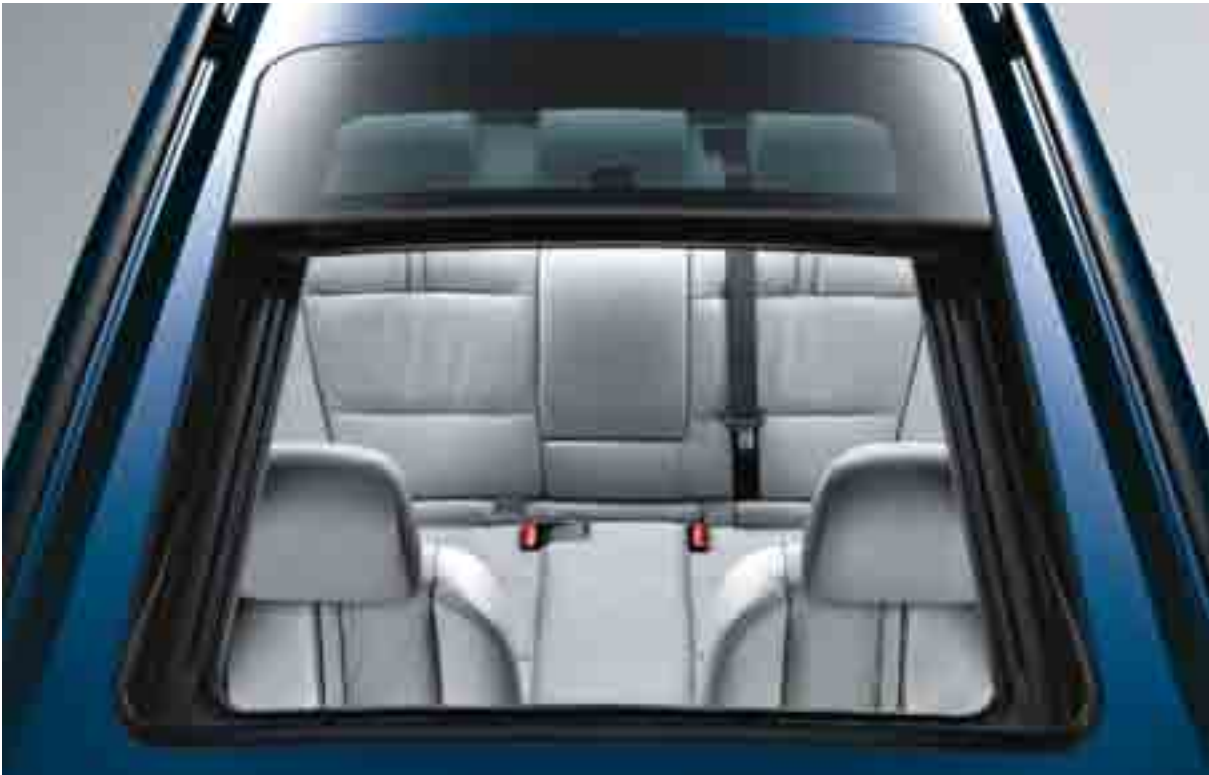
□ Dual-glass-panel Panoramic moonroof features fully electric slide and lift control. Includes trap release, comfort opening/closing function, a wind deflector to help keep the wind out, and an electric sun shade to help shield cabin from excessive heat. (Included in Premium Package.)
