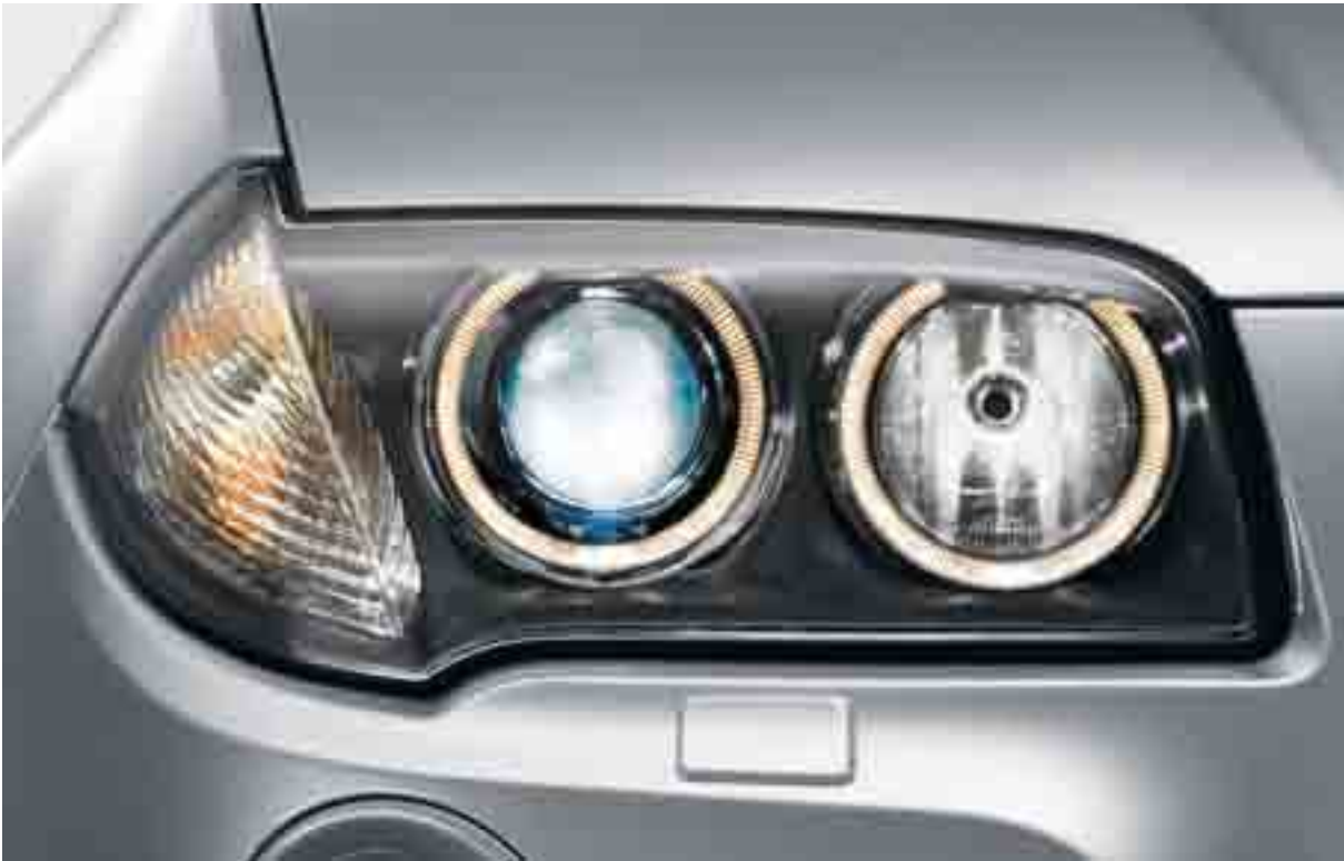
□ Xenon Adaptive Headlights optimize road illumination when the X3 enters a curve or bend, helping to enhance safety when driving at night. Sensors continuously monitor the angle of the steering wheel, the vehicle's speed, yaw and other factors to determine the direction in which the X3 is heading. The headlights swivel accordingly, up to 15 degrees left or right. Xenon low- and high-beam headlights illuminate the road ahead and to the side with brilliant clarity. Includes auto-leveling to adjust for varying passenger and cargo loads. The Corona headlight-rings that circle both headlights and high beams also act separately as Daytime Running Lights and parking lights. (Shown with optional Cold Weather Package.)
