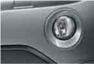
■ Halogen free-form foglights are cleanly integrated into the front air dam, illuminating the road ahead in bad weather and poor visibility.
