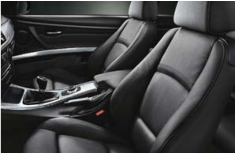
Eight-way adjustable front sport seats make the driving experience more enjoyable. Side bolsters can be power-adjusted to fit your back comfortably while helping to hold you firmly in place during cornering. Includes two-way manual headrests and thigh support.
