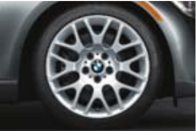
Cross Spoke (Style 197) light alloy wheels with run-flat 2 performance tires . 3 In front: 18 x 8.0 wheels with 225/40 tires; in back: 18 x 8.5 wheels with 255/35 tires. (328i Sport Package; optional on 328i xDrive, requires Sport Package.)
