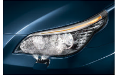
Retractable high-intensity headlight washers help keep lights clear of ice, mud, road salt and other coatings, for maximum road lighting and enhanced driving safety.
