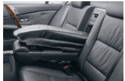
Ski bag allows clean and secure transport of up to four pairs of skis and ski poles. When not extended for use, the ski bag can be stored in the seat, and the center armrest can be left down for use, or folded up to create a third seat.
