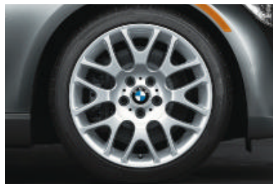
□ Cross Spoke (Style 197) light alloy wheels and run-flat 1 performance tires. 2 In front: 18 x 8.0 wheels and 225/40 tires; in back: 18 x 8.5 wheels and 255/35 tires. (included in 328i Sport Package)
