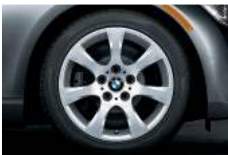
■/□ 17 x 8.0 Star Spoke (Style 185) light alloy wheels with 225/45R-17 run-flat 1 all-season tires. (std. on 335i; included in 328xi Sport Package)
