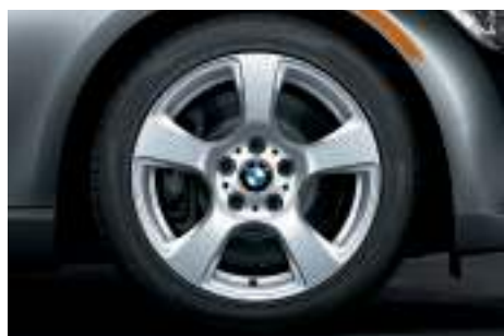
■ 17 x 8.0 Star Spoke (Style 157) light alloy wheels with 225/45R-17 run-flat 1 all-season tires. (std. on 328i/328xi)
