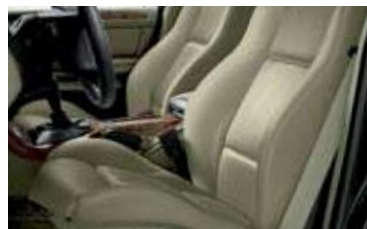
Sport front seats are designed to hold you tight in curves during sporty driving. Seats are eight-way power adjustable with a two-way manually adjustable thigh support. (Included with Optional Sport Package)
