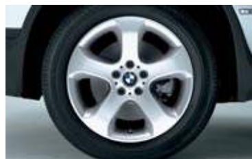
19 x 9 front / 19 x 10 rear Star Spoke (Styling 132) cast-alloy wheels and 255/50R-19 front, 285/45R-19 1 rear performance tires. (opt. with X5 4.4i Sport Package only; performance tires not recommended for winter driving.)
