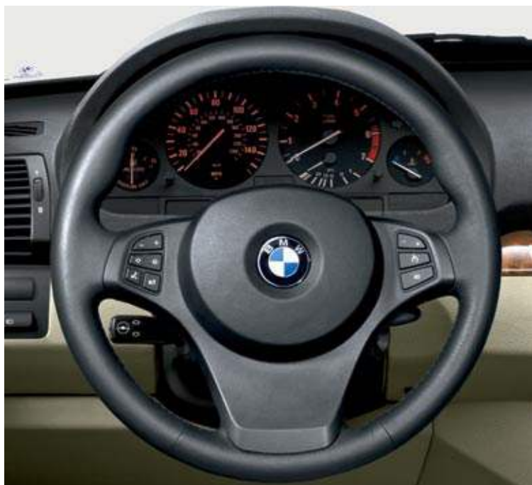
Three-spoke leather-wrapped sport steering wheel features power tilt/telescoping and controls for cruise, audio and (accessory) phone. (Included with Optional Sport Package)
