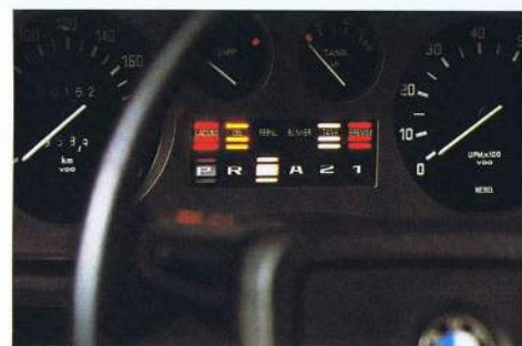
Automatic transmission indicator strip showing position of selector lever (standard on BMW 3.3 Li, otherwise as optional extra).
