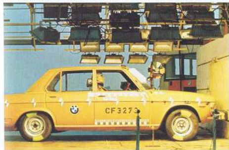
Crash tests to give optimum front and rear collapsing zones.
