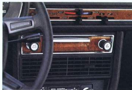
Heating and ventilating system. A powerful 3-speed blower acts as an effective back-up to the modern dual circuit system.
