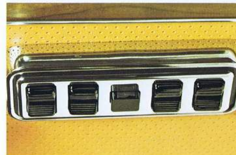
Electric windows. Central control panel for all 4 doors on the driver's door. (Standard on BMW 3.3 Li, otherwise on request.)
