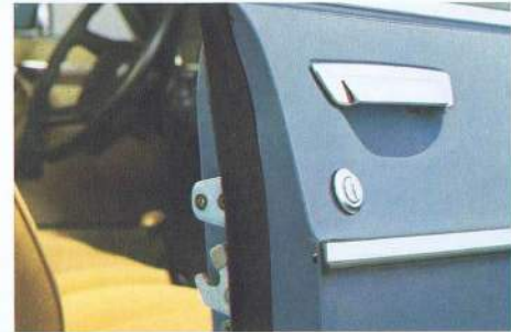
BMW door lock with ball catch and safety anti-burst strikers — do not open on impact.
