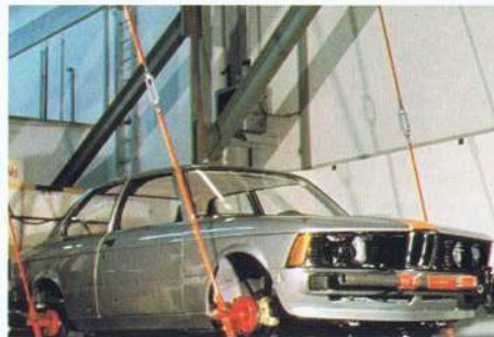
Simulating collisions at slow speeds with a pendulum.
