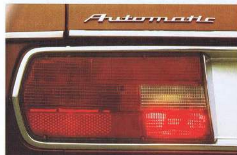
Tail fog light integrated into rear lights.
