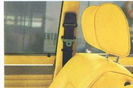
Systematic safety thanks to the standard combination of head restraints (angle adjustable) and inertia reel seat belts.
