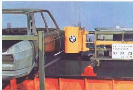
Checking door stability.
