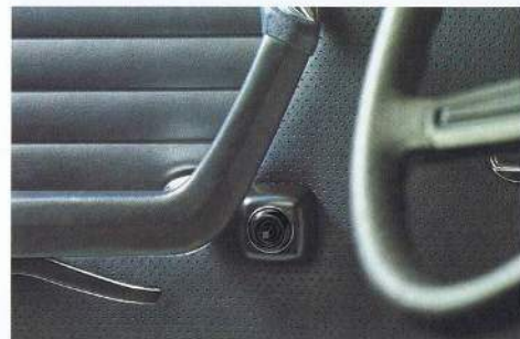
Wing mirror adjuster. Control lever in a protected position on the inside of the driver's door.
