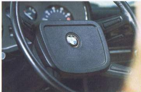
Foam-padded 4-spoke safety steering wheel with large central boss.
