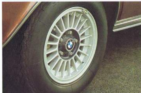
Light alloy wheels reduce the amount of unsprung mass and increase active safety (standard on BMW 3.3 Li, otherwise as optional extra).
