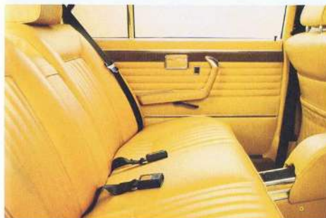
3-point inertia-reel safety belts for rear seats and central arm-rest in front. Inertia-reel belts standard on BMW 3.3 Li, optional on other models.
