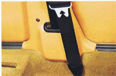
Inertia reel seat belts. Covered reel for the front seat 3-point seat belts.
