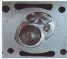
2. The triple hemisphere swirl action combustion chambers achieve optimum mixture distribution and smooth combustion. The result: unique development of power, favourable exhaust ratios and economic consumption.
