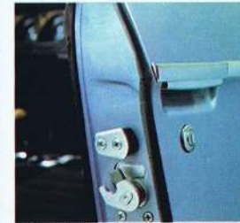
Safety door locks which do not burst open in a collision.
