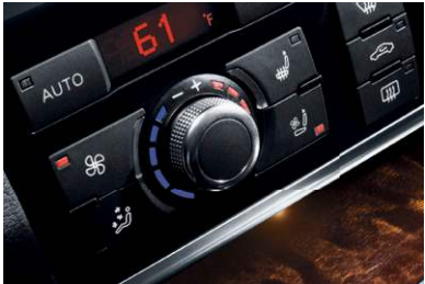
Front seat temperature controls
