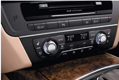
Four-zone automatic climate control
