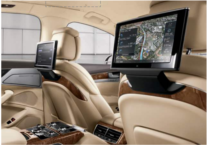
.14 – Rear Seat Entertainment With vibrant dual 10" screens, the available Rear Seat Entertainment option can display a wealth of media choices and information, including navigation. Each rear seat occupant can access their own media controls located on the center armrest.
