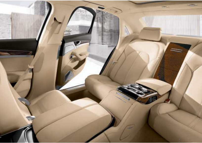
.11 – Executive Rear Seating The available A8 L Executive Rear Seat Comfort package adds a level of personalized comfort to the benchmark in executive luxury. Power rear single seats with massage function immerse you in sumptuous relaxation, while a fixed, leather-covered rear center console and Rear Seat Entertainment system with dual 10" screens create a mobile business or pleasure center. This package also features a small refrigerator between the rear seats as well as rear-seat ventilation.
