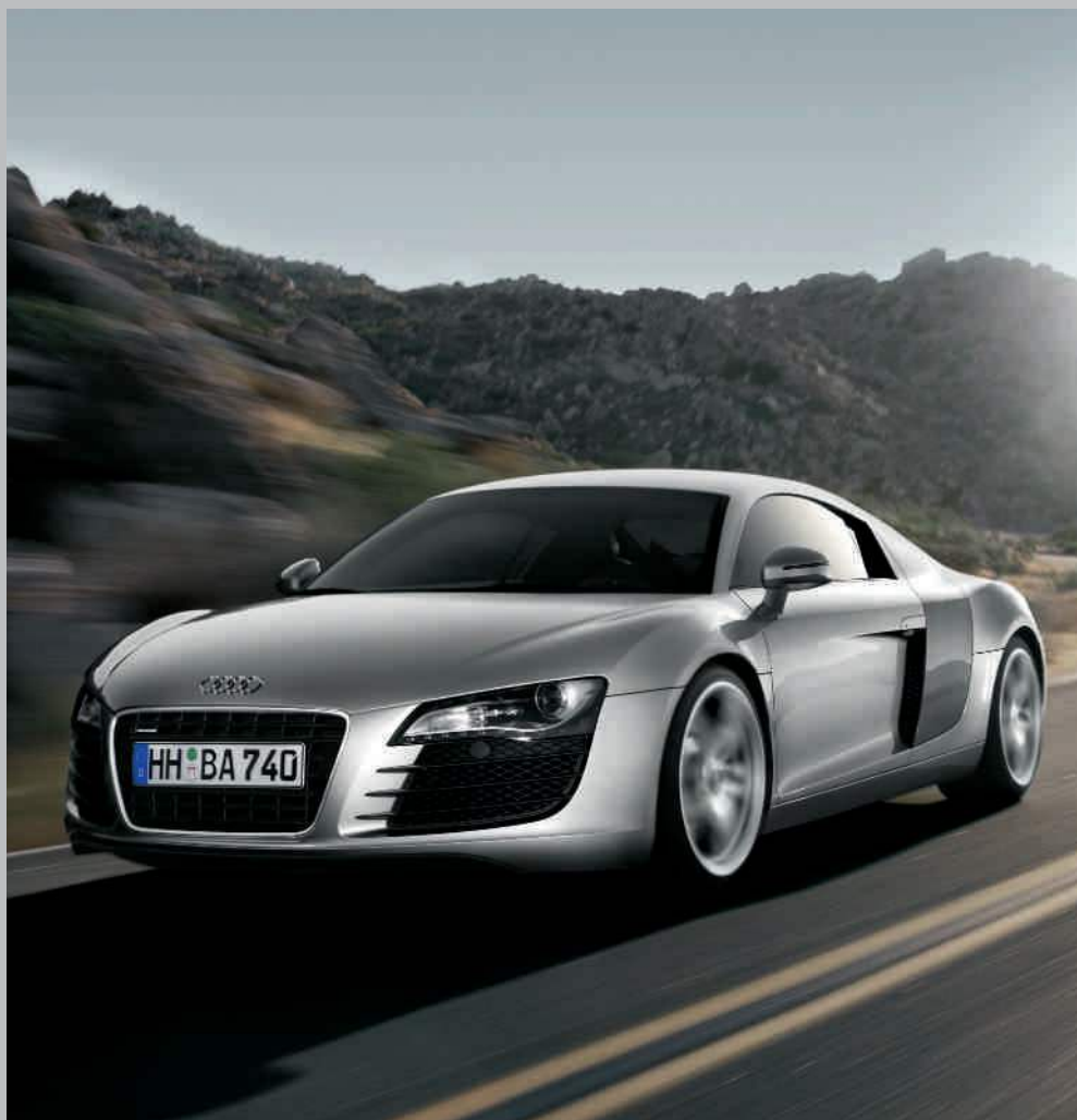
Cast aluminium wheels, 6-arm design size 8.5 J x 18 at front, size 10.5 J x 18 at rear, with 235/40 R 18 tyres at front and 285/35 R 18 tyres at rear. (Standard for R8 4.2 FSI quattro)
