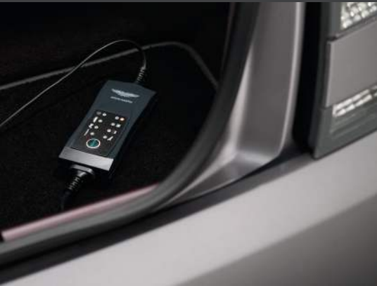
Battery Conditioning Unit
