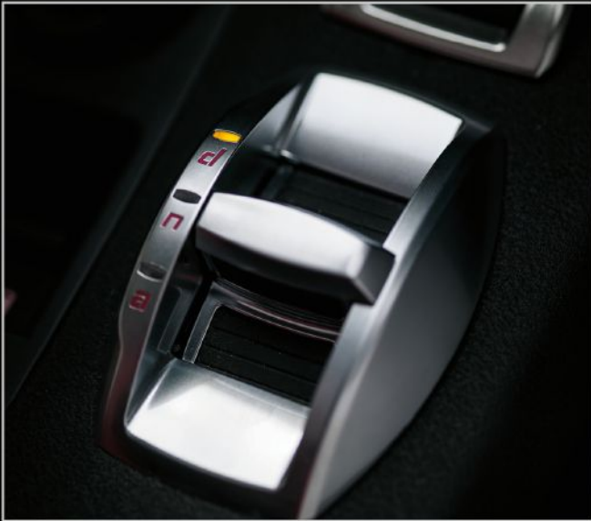
4-position, Alfa DNA driving mode selector
