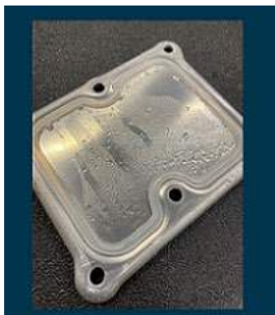
Figure 5: Condensation on high-voltage system connection cover.
