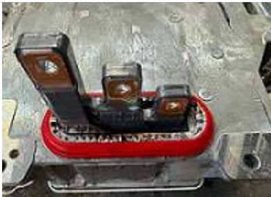
Figure 4: Corrosion on high-voltage system connection for power and control electronics for electric drive.
