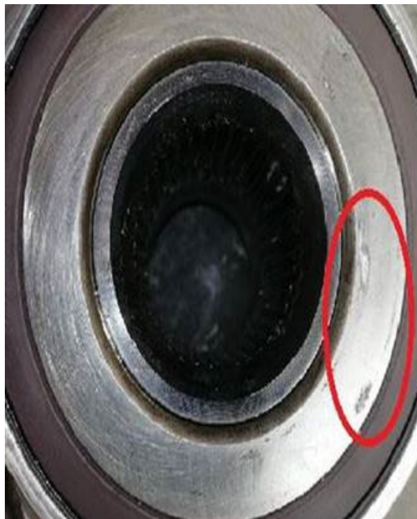
Figure 5: Metallic particles/damage in the wheel hub/bearing.
