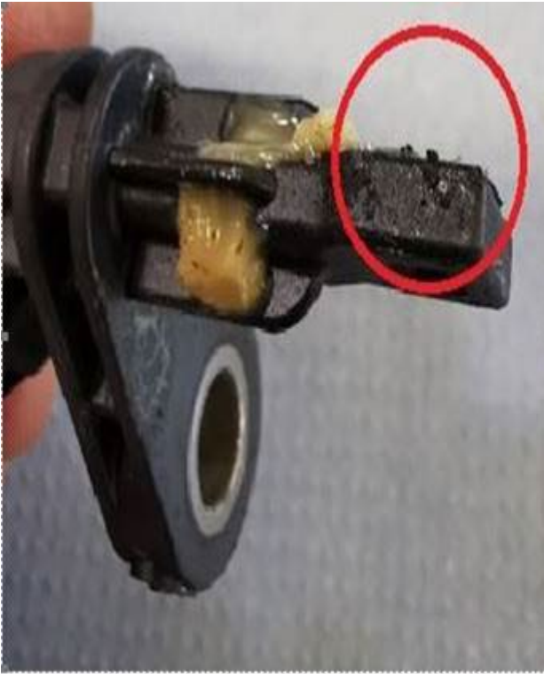
Figure 2: Metallic particles in the speed sensor.
