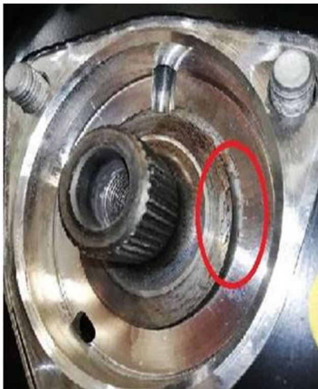
Figure 4: Metallic particles/damage in the wheel hub/bearing.
