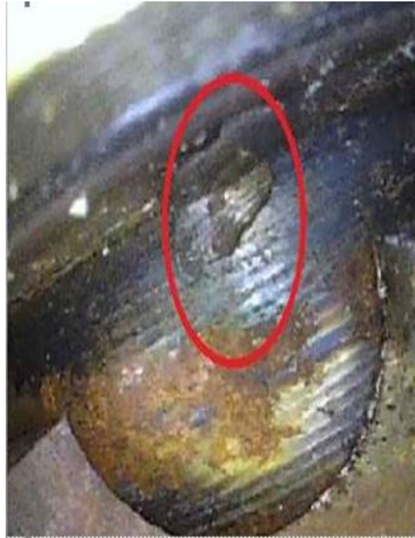
Figure 3: Metallic particles in the hub.
