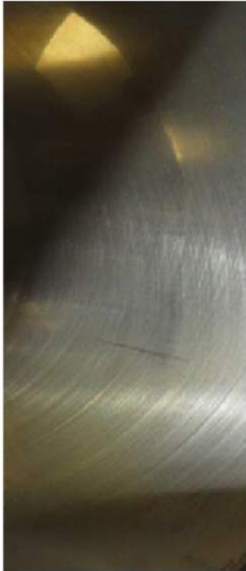
Figure 2 - Showing normal cylinder wall wear
