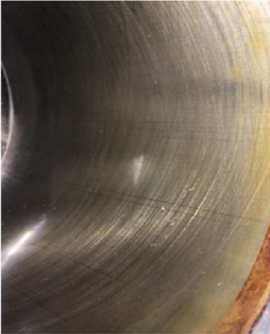
Figure 3 - Showing normal cylinder wall wear
