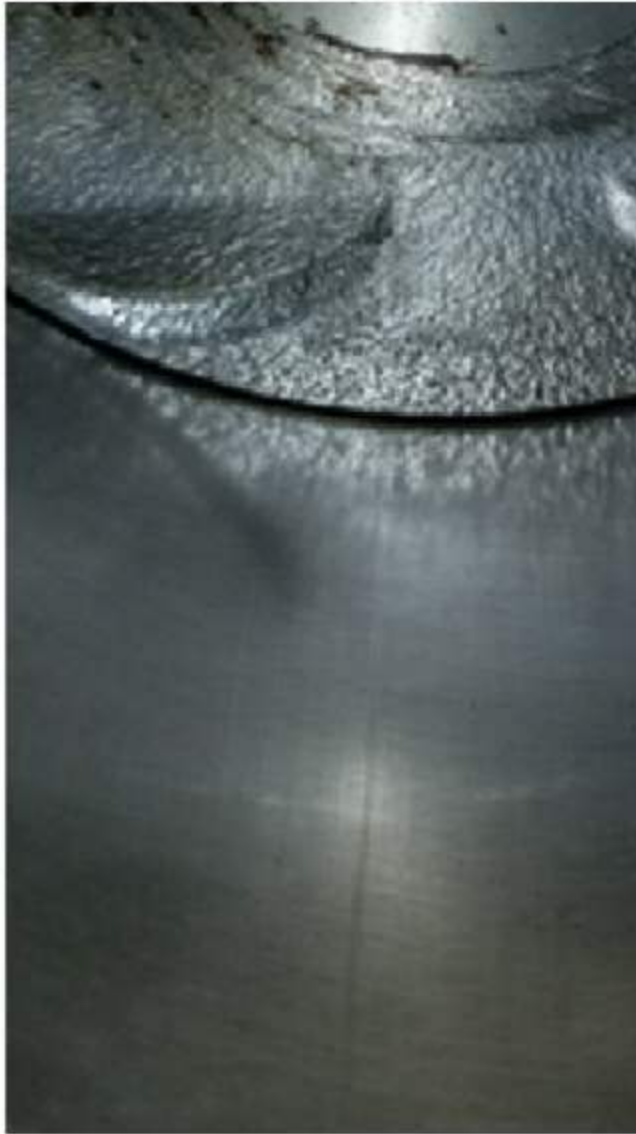
Figure 4 - Showing a damaged cylinder wall
