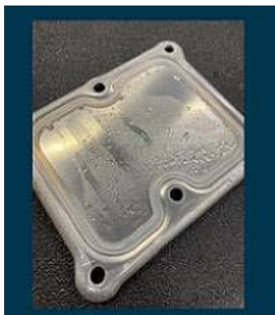
Figure 5: Condensation on high-voltage system connection cover.
