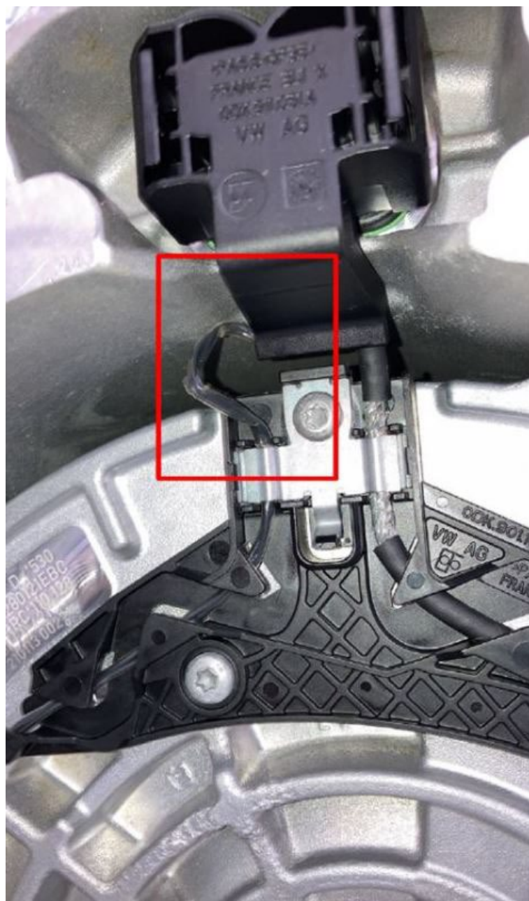
Figure 1. Wire not fitted correctly
