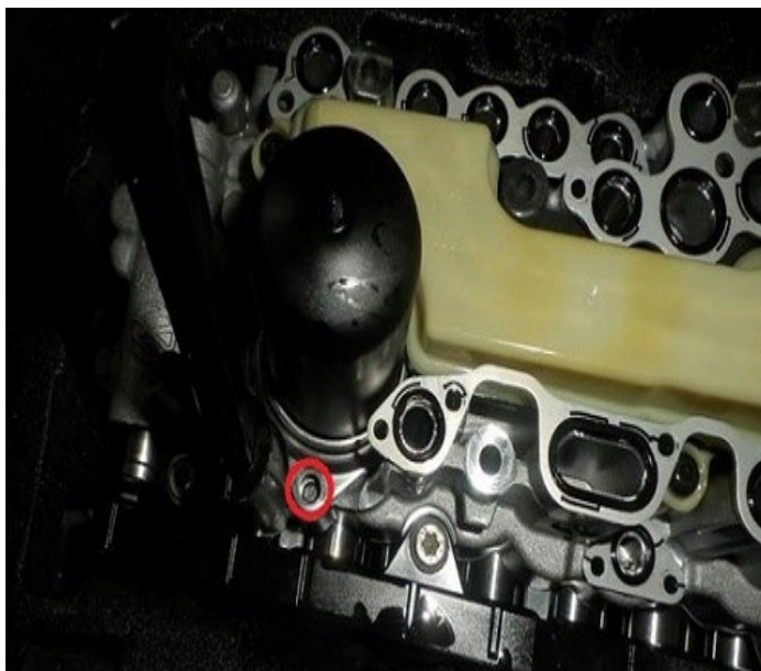
Figure 5. The bolt head is missing.
