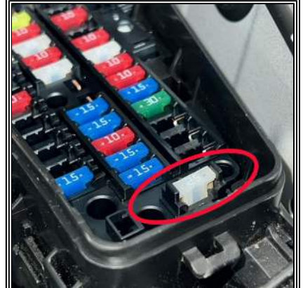
No Good (not secured)
