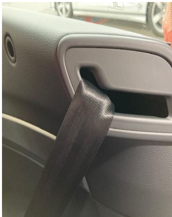
Figure 3. The belt on the edge of the slot that it comes out of.
