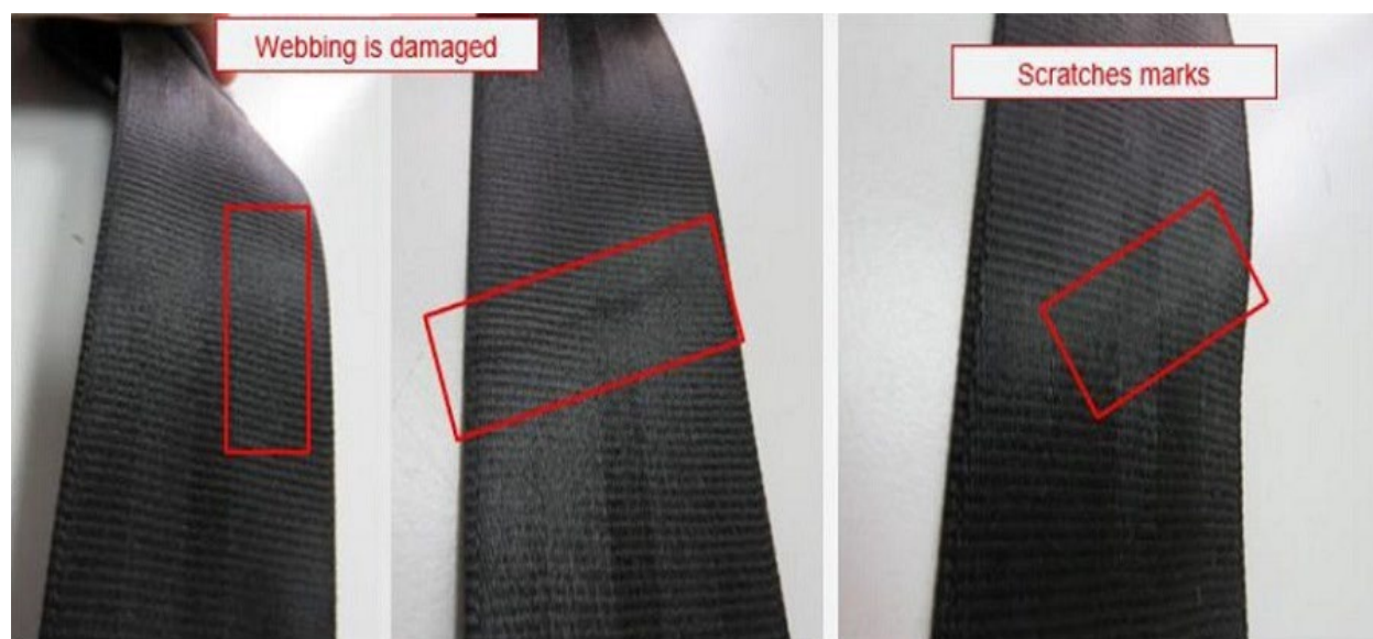
Figure 1. Marks indicating that the belt was trapped in the driver door
