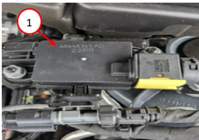
Fig. 1 EGT Sensor Location
