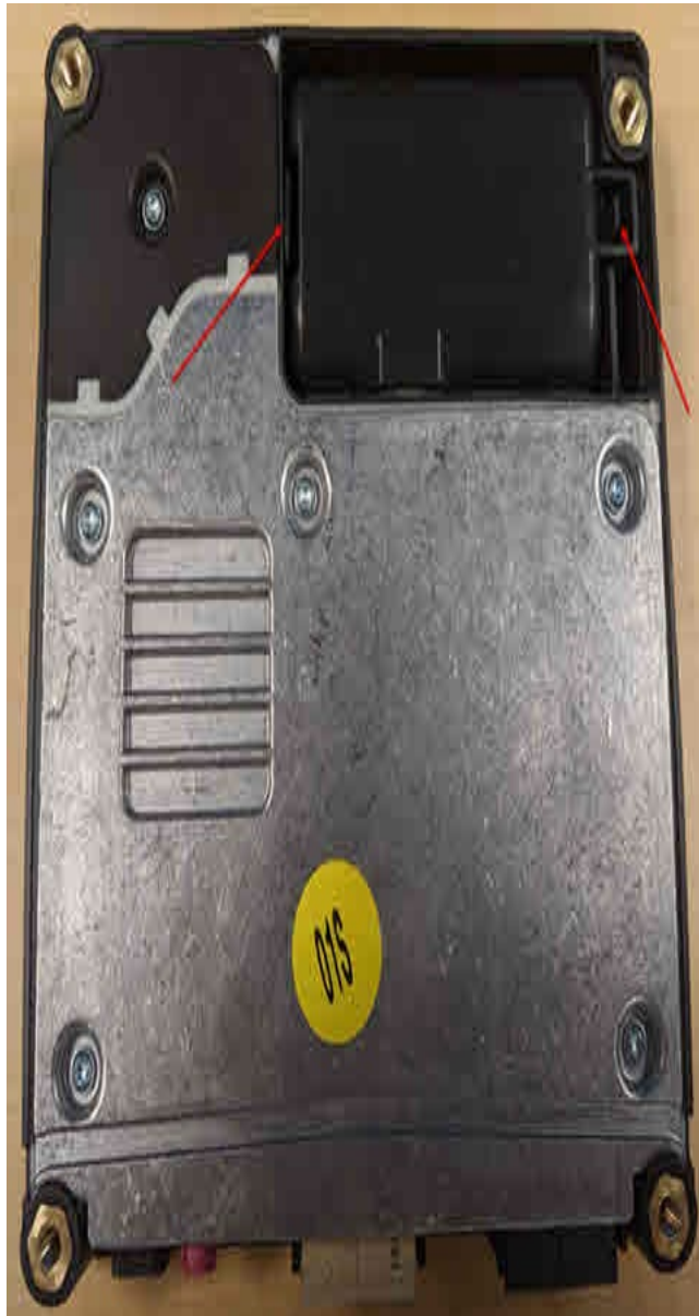
Figure 2. Backup battery compartment location.
