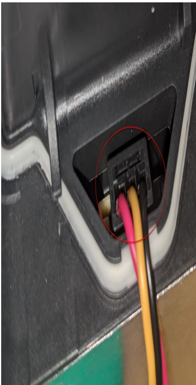
Figure 3. Backup battery connector (no release mechanism).
