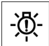
Exterior light warning light
