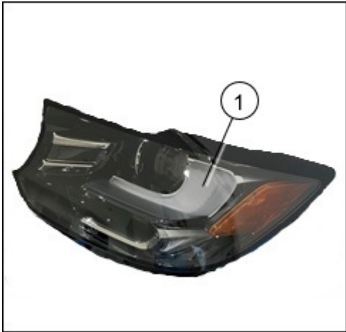
Combination light with AFS (1): Parking light/daytime running light (DRL)
