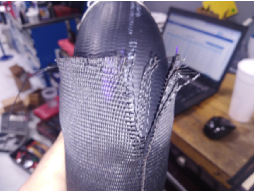
#3 Picture below inside the circled area shows damage to inner hose beneath abrasion sleeve
