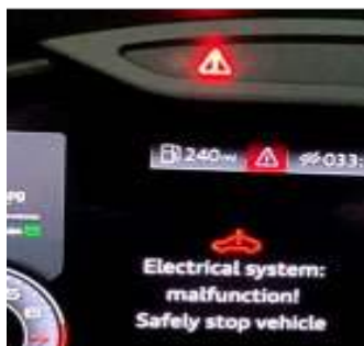
Figure 1. Warning lamp associated with message.
