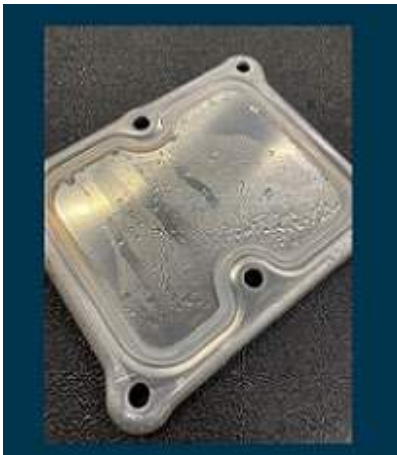
Figure 5: Condensation on high-voltage system connection cover.
