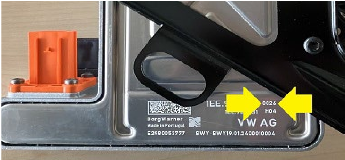
Figure 2. Example of software version number (0026) on label/embossing on high-voltage heater Z132
