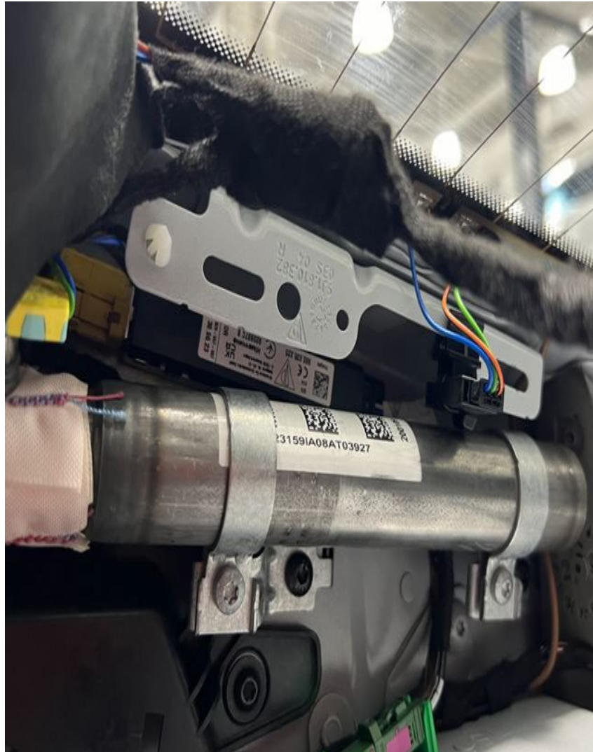
Figure 5: Insulate connector and harness.
