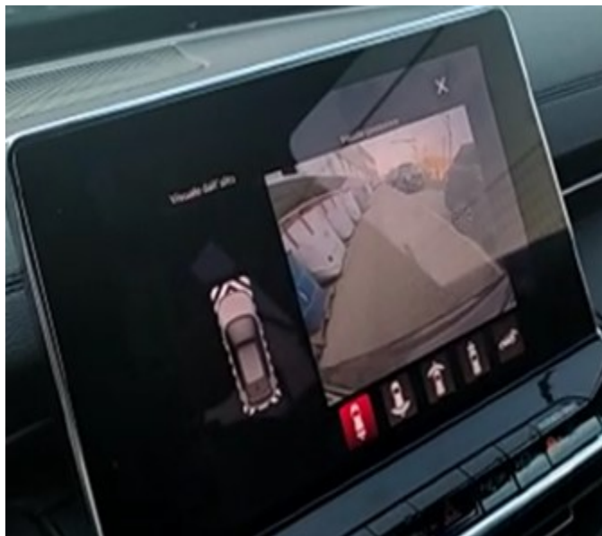
Fig. 1 Missing Gridlines When In Reverse Gear
