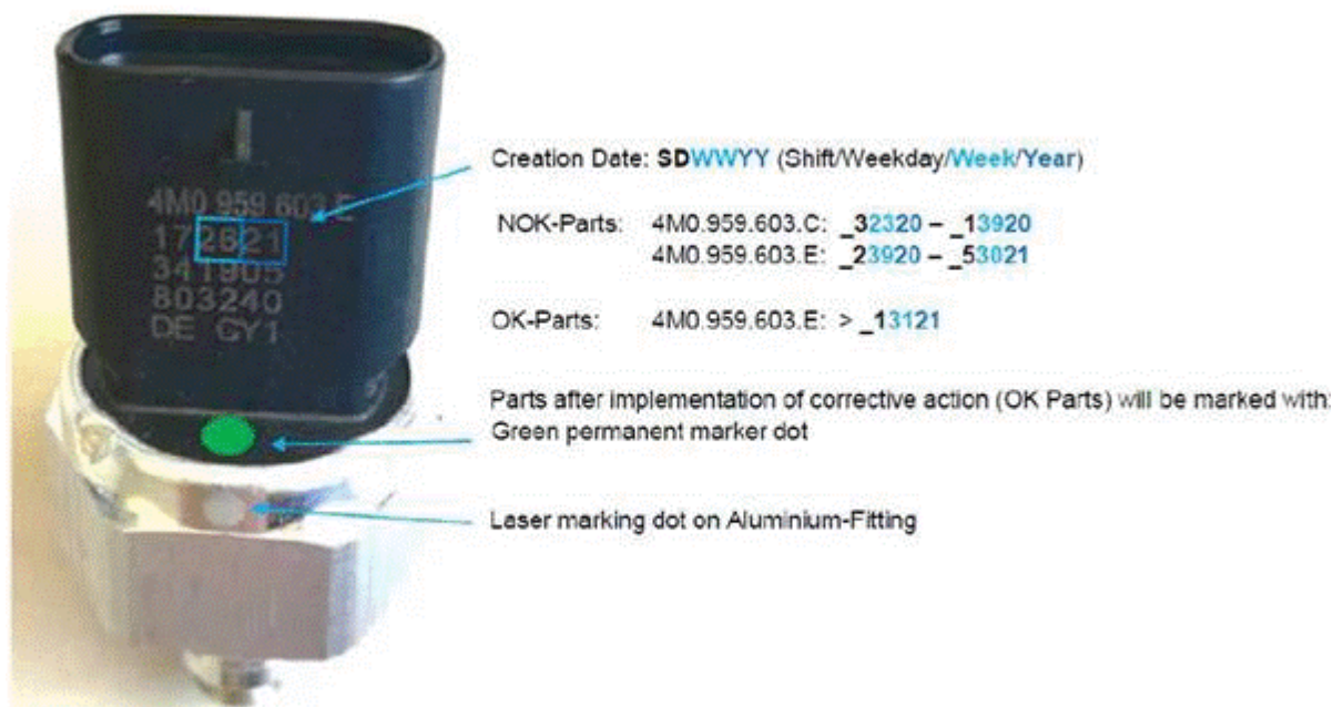
Figure 1. Pressure and temperature sensor markings and build date
