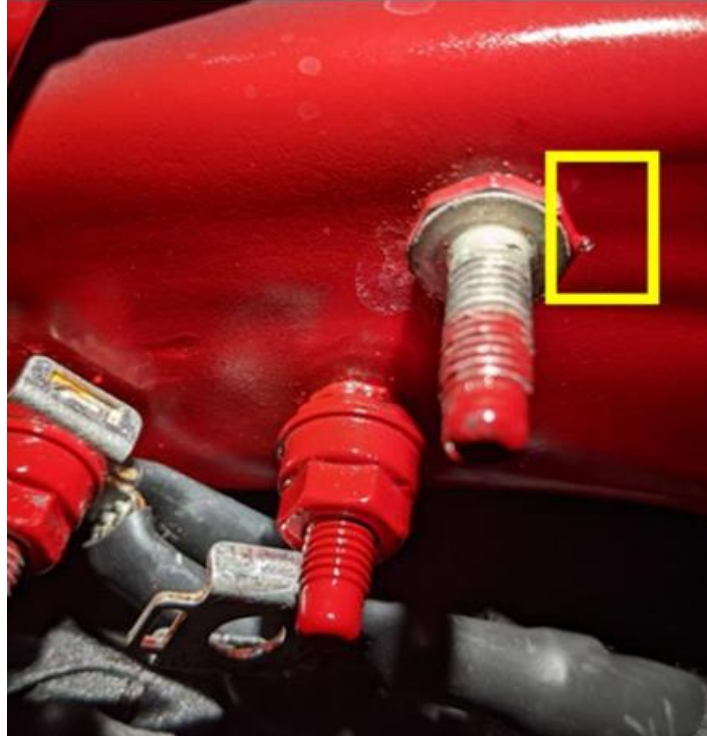
Fig 3. Weld slag to be filed or ground down.
