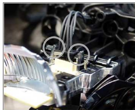
Example of an incorrectly secured plug connection
