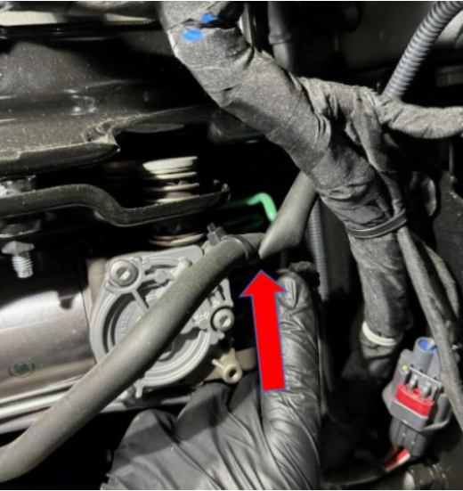
Example of twisted hoses on the 2024 Hummer EV
