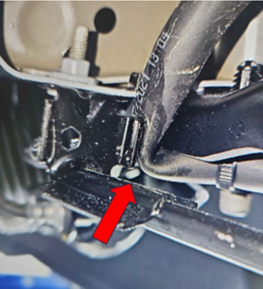
Example of a pinched hose on a 2023 Cadillac Escalade below:
