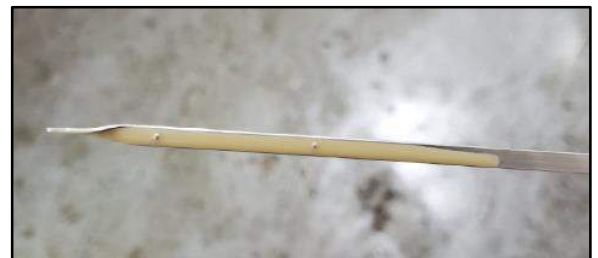
Figure 2. Engine Oil (Milky/Discolored)
